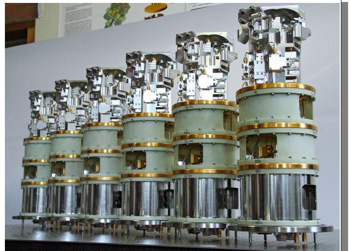
Figure 21: Six of the 64 ALMA Band 9 cartridges, a main part of the Dutch contribution to the ALMA project, designed and produced in a collaboration between NOVA and SRON. Credit: NOVA/SRON
