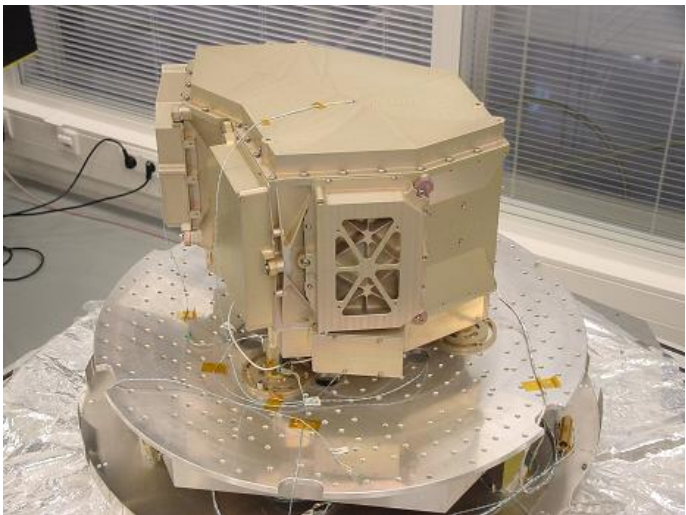
Figure 22: The MIRI spectrograph optics for the JWST satellite in the NOVA OIR Group lab at ASTRON. Credit: NOVA
