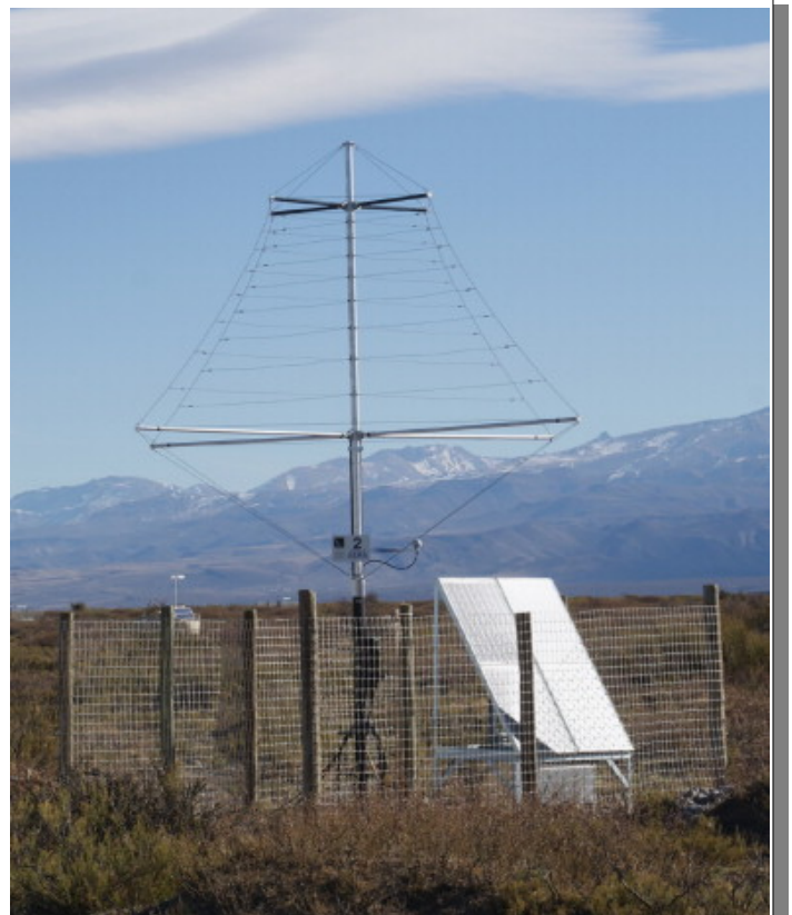
Figure 12: An AERA station at the Pierre Auger Observatory, an example of a cross-discipline initiative to detect ultra-high-energy cosmic rays using radio astronomy techniques. Credit: IMAPP/RU Nijmegen
