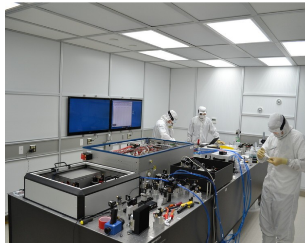
LIGO Hanford Pre-Stabilized Laser in Clean Room Enclosure
