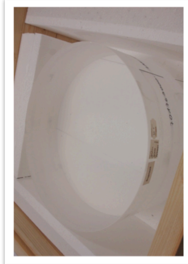
AdV test mass substrate
