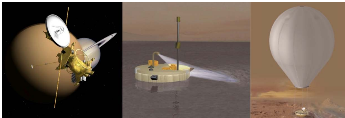
FIGURE 8.13 The three elements of the 2009 TSSM mission architecture: A Titan orbiter, a lake lander, and a hot-air balloon. SOURCE: ESA/NASA;
