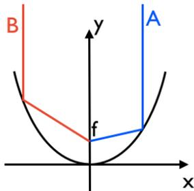
In the limit of long  $f$ -ratios, the shape of a paraboloid can be approximated by a spherical surface. This has the advantage that spherical surfaces are easier (and therefore cheaper) to produce, and do not suffer from coma.
