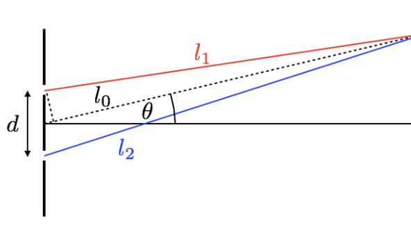
We make use of the *Fraunhofer approximation*, which simply means that we assume that the distance between the slits and the screen is very large compared to the separation between the slits ( $l_0 \gg d$ ), so that the light “rays” along  $l_1$  and  $l_2$  can be considered parallel. (In a real telescope, this is still a valid approximation due to the focussing of the light by a lens or mirror.)
