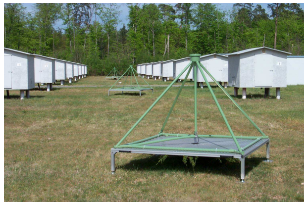
FIG. 1: Inverted V dipole antenna for the LOPES experiment integrated into the KASCADE array. Only two 'legs' of the dipole are equipped with antennas, such that only one polarisation in east-west direction can be measured. In the background one can see some scintillator sampling detectors in wooden housings on the campus of the Forschungszentrum Karlsruhe.
