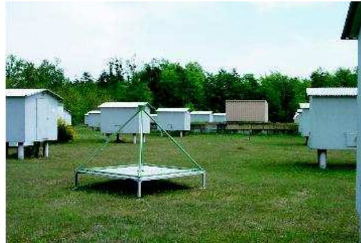
Figure 7. Dipole radio antenna in the Field Array of KASCADE. A Grande station on top of the Muon Tracking Detector is also seen.
