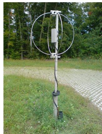
(b) Small Aperiodic Loaded Loop Antenna
