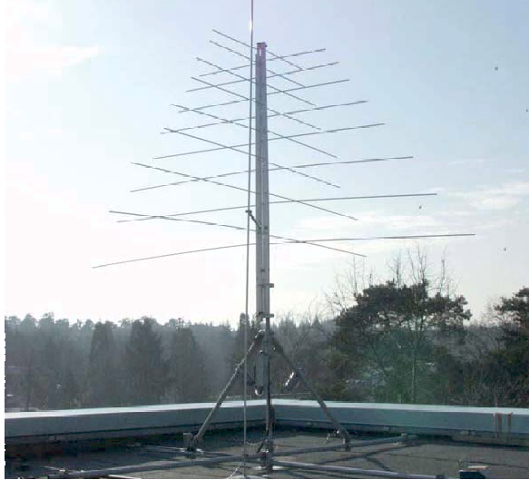
Figure 15: Logarithmic periodic dipole antennas used for LOPES STAR optimized for the frequency band from 40 to 80 MHz and azimuth angles smaller than 80^\circ .
