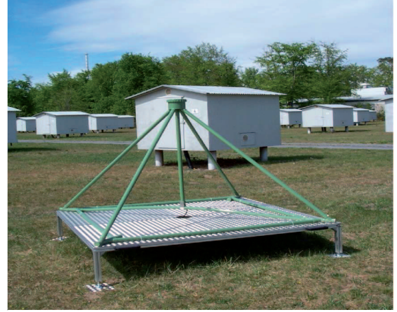
Figure 7: V-dipole antenna as used in LOFAR and LOPES. The length of the arms are 1 m.
