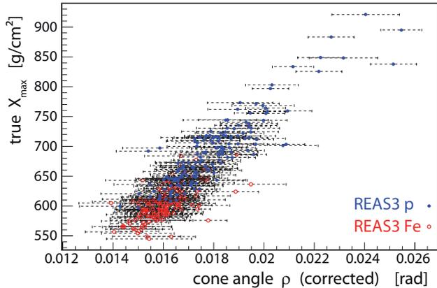
Figure 3: Correlation of the cone angle  $\rho$  of REAS3 proton and iron simulations with the true  $X_{\max}$ , after correcting  $\rho$  for its zenith angle dependence.
