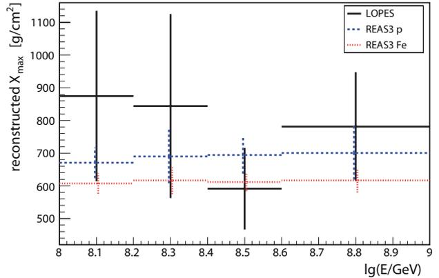
Figure 5: Reconstructed  $X_{\max}$  (mean and standard deviation) for the LOPES measurements and the REAS3 proton and iron simulations using the calibration constant  $c_\rho$  determined with the simulations.
