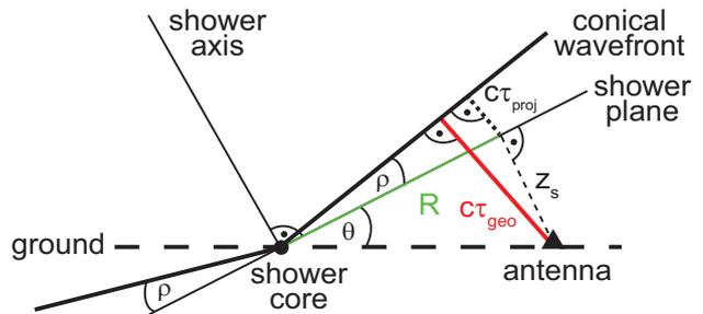
Figure 2: Sketch of conical wavefront with a cone angle  $\rho$ : the pulse arrival time in an individual antenna is delayed with respect to a plane wavefront since the geometrical delay  $\tau_{\text{geo}}$  is enlarged. It depends on the lateral distance  $R$  of the antenna and the antenna height in shower coordinates  $z_s$ . Correcting for the shower geometry, one obtains the projected geometrical delay  $\tau_{\text{proj}}$ .  $c$  is the speed of light,  $\theta$  the zenith angle.
