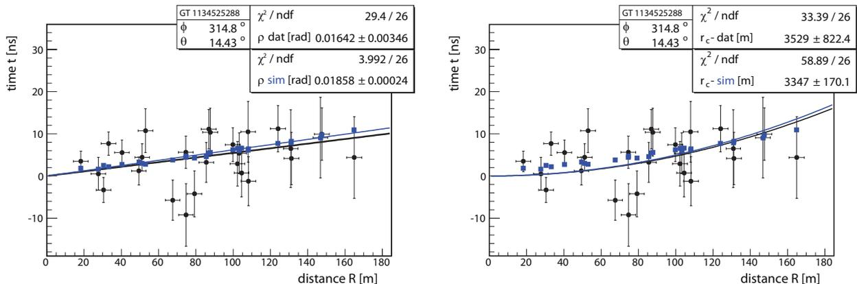
Figure 1: Example event for wavefront reconstruction (LOPES measurement: circles with error bars, REAS3 simulations: squares). Plotted are the pulse arrival times in the individual antennas corrected for the shower geometry ( $\hat{=} \tau_{\text{proj}}$  in figure 2). A plane wavefront would correspond to a horizontal line at 0 ns. The same event is plotted twice, fitting a conical wavefront with a cone angle  $\rho$  (left) and a spherical wavefront with a curvature radius  $r_c$  (left).
