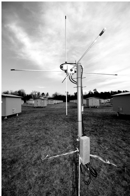
Figure 1: Picture of the tripole, the new antenna type used at LOPES 3D. The metal box at the pole is the housing for the preamplifier.
