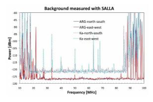
Fig. 1: Measured radio background at Karlsruhe (dashed line, Ka) and at Pierre Auger Observatory, Argentina (solid line, Arg). The differences in the background are due to overload protection outside the shown measuring range.
