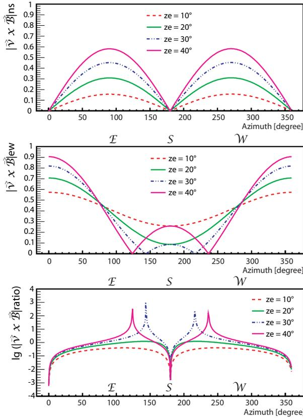
Fig. 4: Relative contributions of the  $\vec{v} \times \vec{B}$ -vector for the polarization components north-south (top panel), east-west (middle panel), and their ratio (bottom panel) vs. the azimuth angle calculated for different zenith angles.
