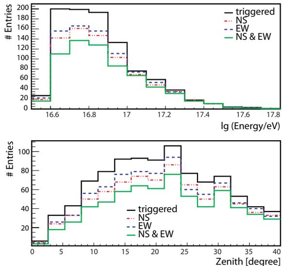
Fig. 2: Primary energy and zenith angular distributions of the triggered (by KASCADE) and of the radio (by LOPES) detected events.
