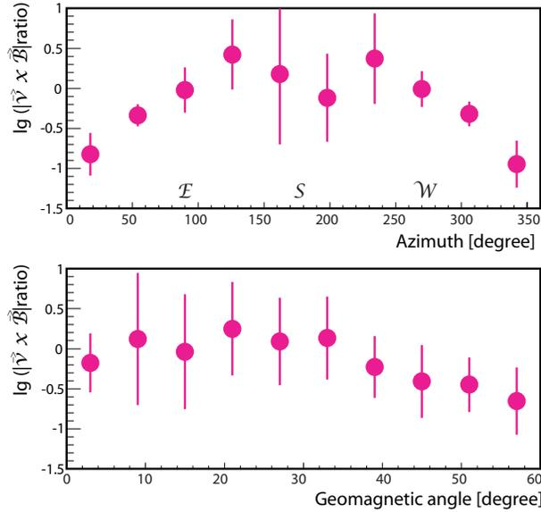
Fig. 6: Ratio of the north-south divided by the east-west component of the  $\vec{v} \times \vec{B}$ -vector for the measured events taking into account the geometry of the shower axis only vs. the azimuth angle (upper panel) and the geomagnetic angle (lower panel) of the shower. Mean values and spread of the distributions are shown.
