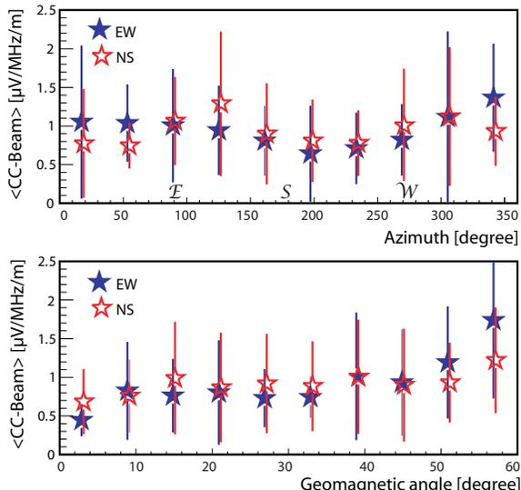
Fig. 3: The normalized CC-Beam values for both polarization components vs. the primary azimuth angle (top panel) and geomagnetic angle (bottom panel). Only events with an estimated primary energy  $> 10^{16.9}$  eV are used. Mean values and spread of the distributions are shown.
