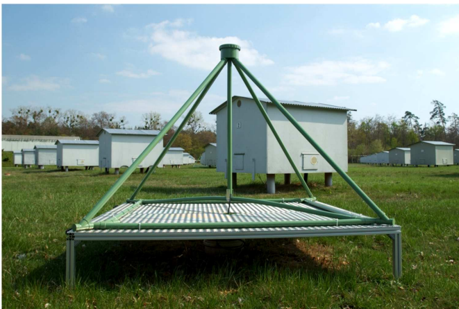
Figure 2: LOPES inverted V-shape dipole antenna.
