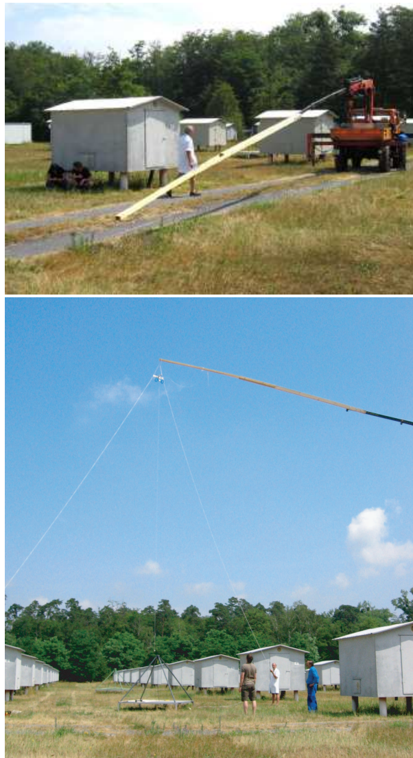
Figure 4.4: Calibration campaign at the LOPES field. Top: Preparation of the setup, like mounting the wooden beam. Bottom: Configuration during the actual measurement.
