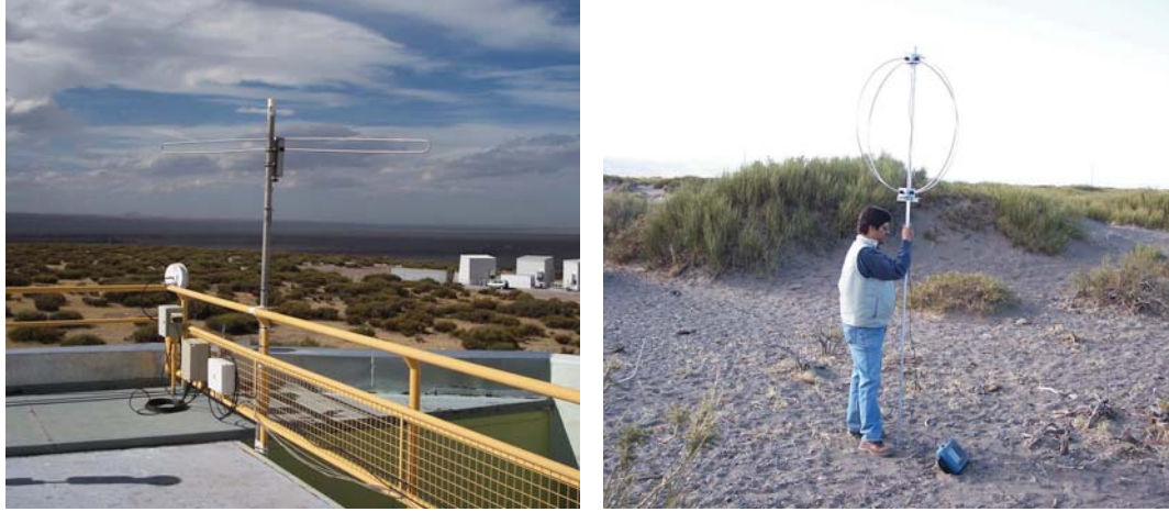
Figure 5.1.: Left: preliminary test beacon at the roof of Coihueco; right: measurement of the beacon power at the AERA site with a mobile, 1 m diameter SALLA on a 3 m pole and a spectrum analyzer.
