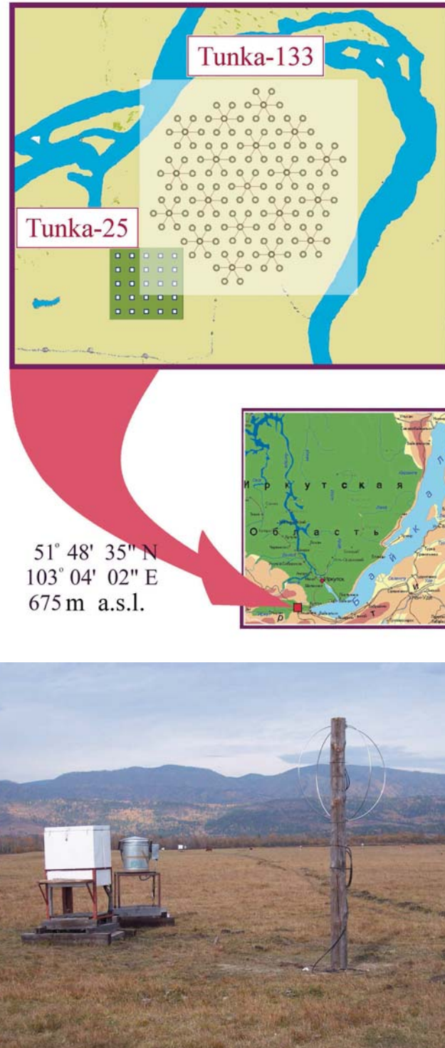
Figure A.1.: Top: Map of the Tunka experiment with a hexagonal structure of photomultiplier detectors for Cherenkov light emitted by air showers [144]. It covers an area of \sim 1 \text{ km}^2 . Bottom: SALLA installed at Tunka cluster 7, cluster DAQ electronics box (white box), and central photomultiplier detector.
