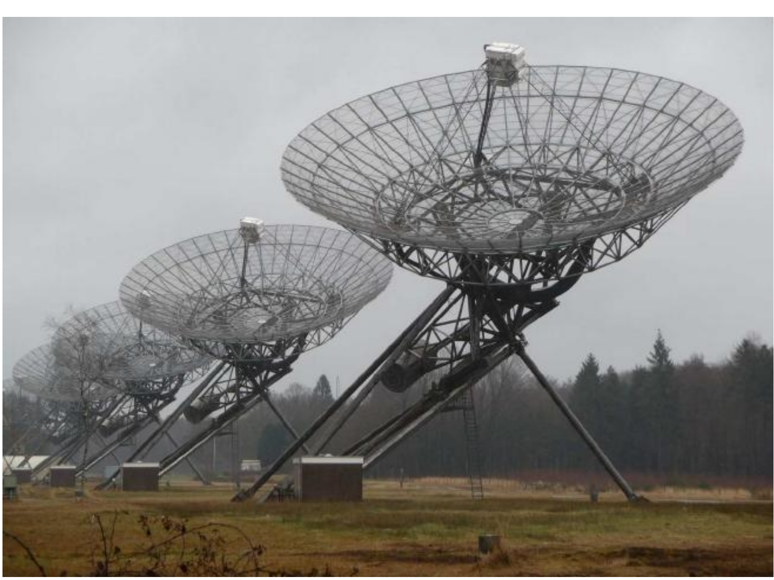
Westerbork Synthesis Radio Telescope (WSRT) in Drenthe - 14 dish-shaped antennas with a diameter of 25 meters each; observing frequencies between 120 MHz - 8.3 GHz
