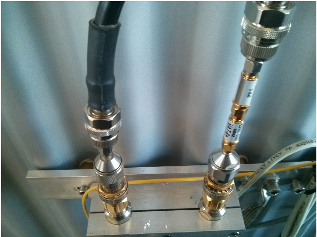
Figure 7: Close up image of the attenuators with the attenuator for the left signal path removed.
