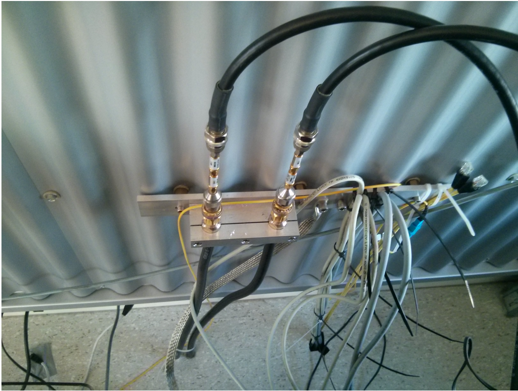
Figure 6: Image of the two signal attenuators in the signal path.
