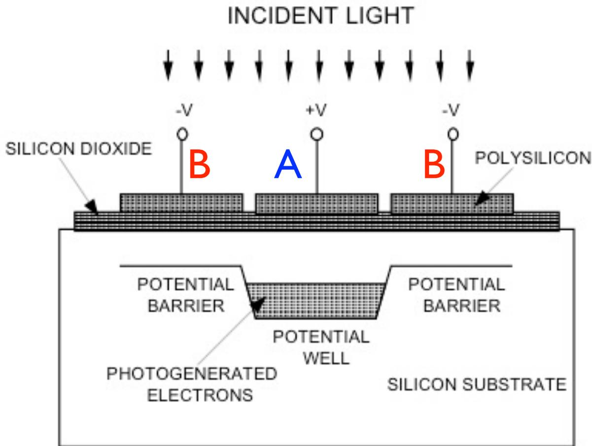
Schematic illustration of a single CCD pixel
