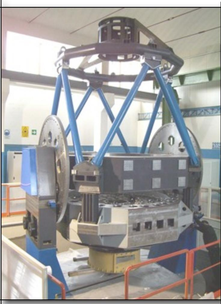
OmegaCam on the ESO 2.6 m VST (“VLT survey telescope”):
