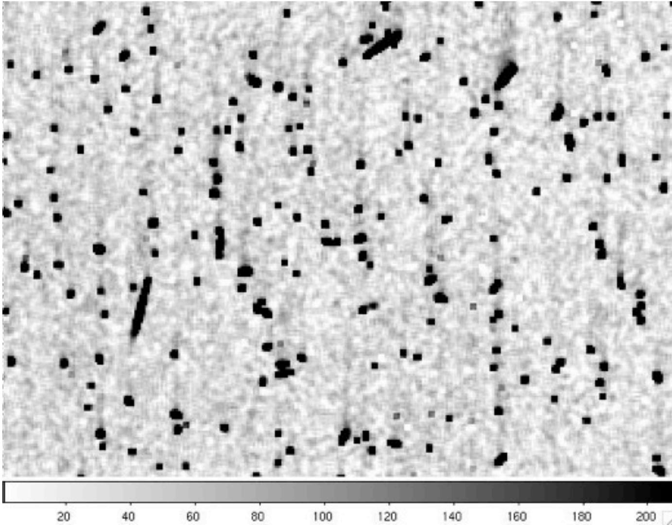
Note the vertical “trails”: Charge “left behind” during CCD read-out
