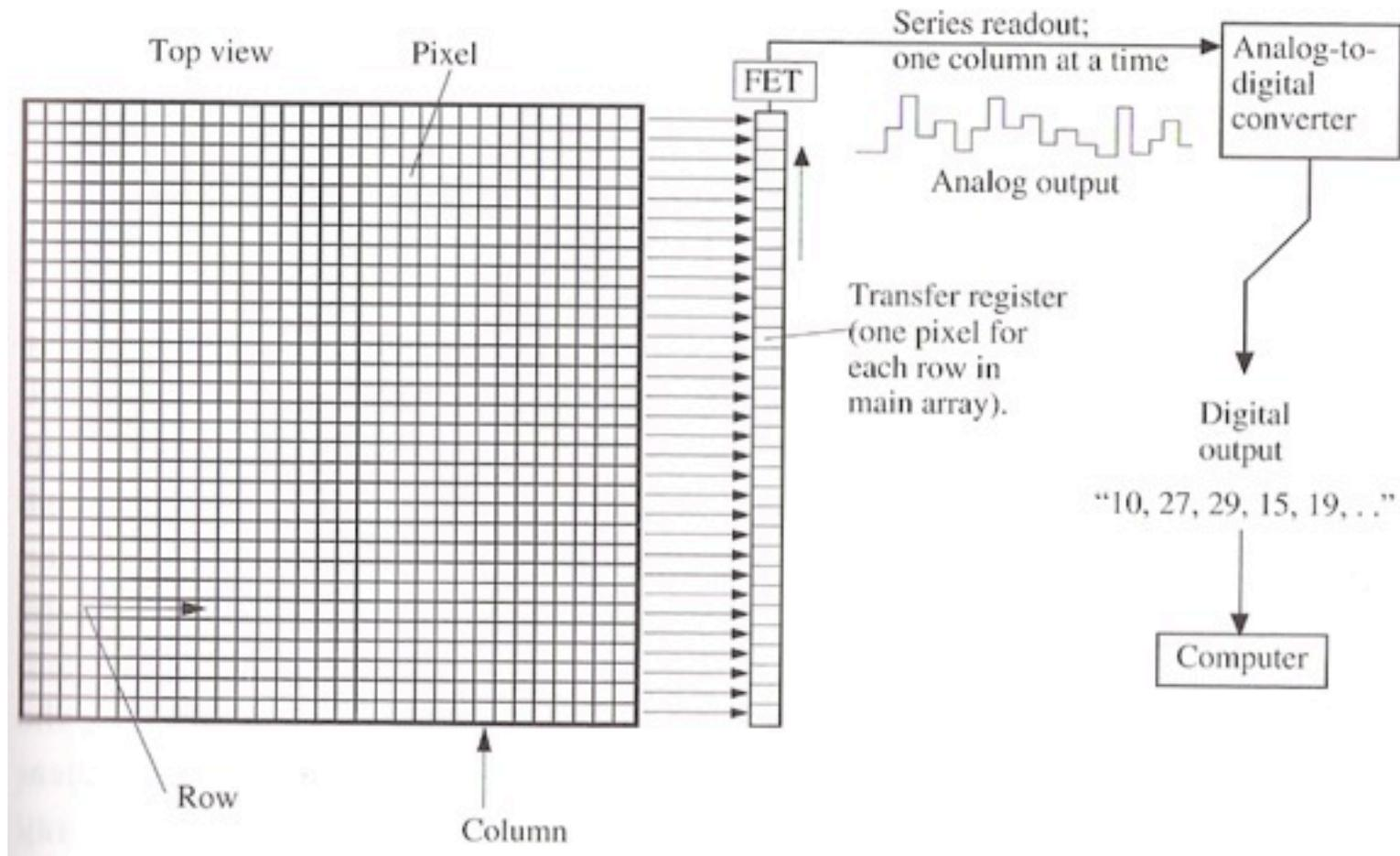
CCD “read out” one column at the time, pixel by pixel. Charges converted to a voltage and then to 16-bit “Digital Numbers” via an analogue-to-digital converter.
