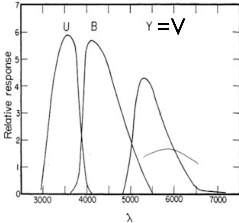
FIG. 1.—Response of the photometer to equal energy at all wave lengths
