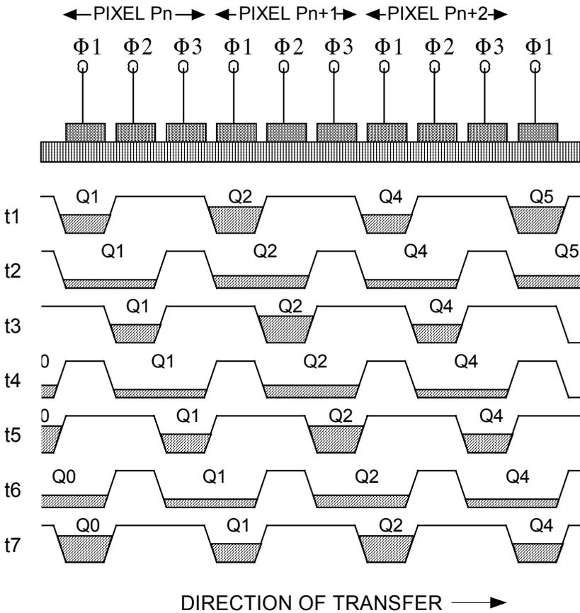
At the end of the exposure, the charges are shifted across the CCD by cycling the voltages on electrodes.
